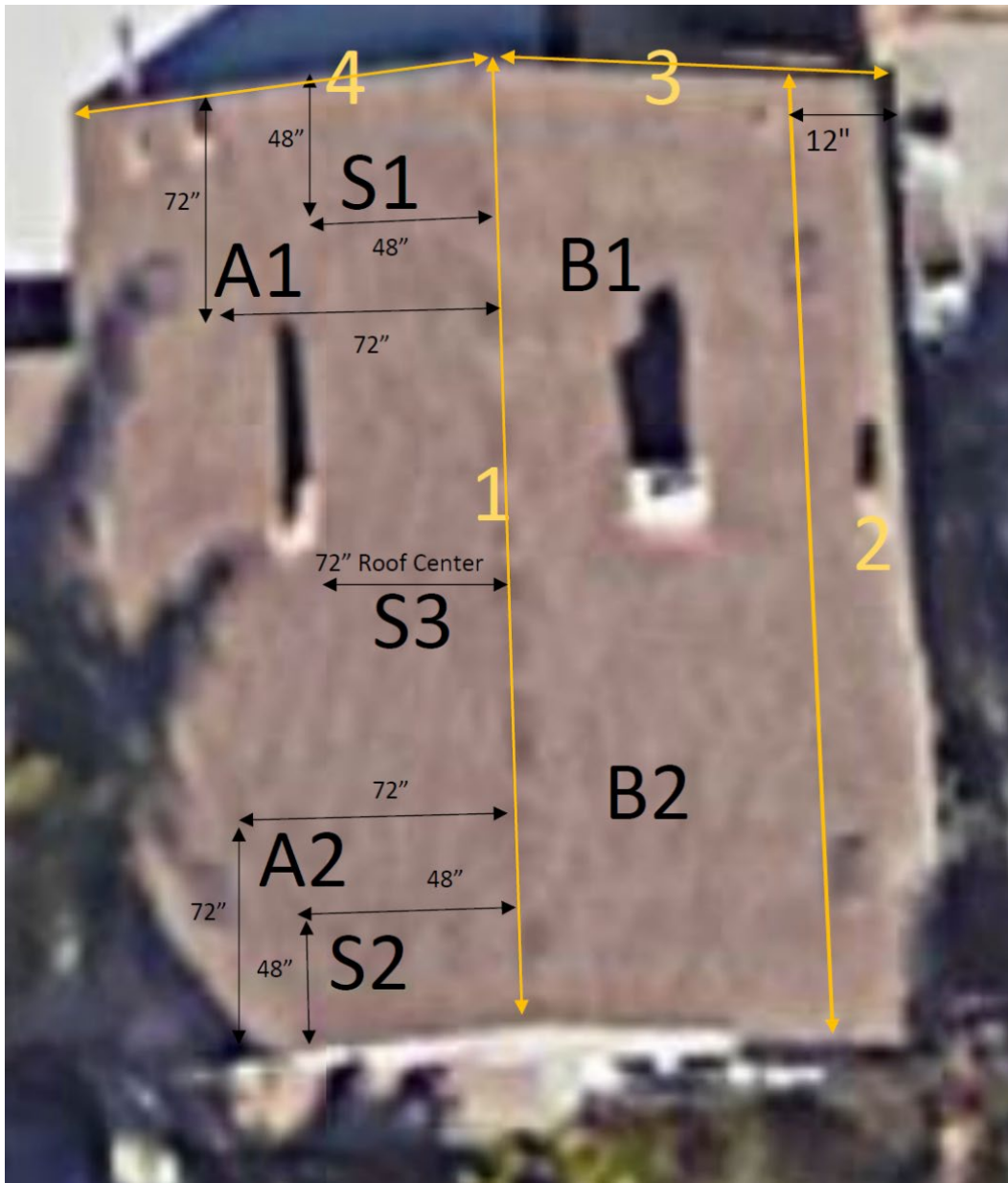
Figure 2-1: PVEL annotated satellite image of a sample roof in the study. Numbered yellow lines indicate distance measurements; A1, A2, B1, and B2 denote slope measurements. Imagery source: Google Earth.
